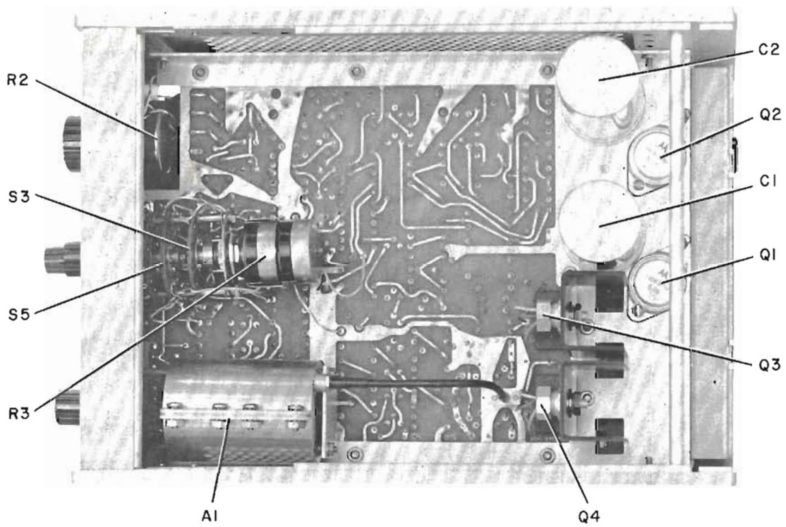
Figure 8-5. Chassis Component Identification - Top View
