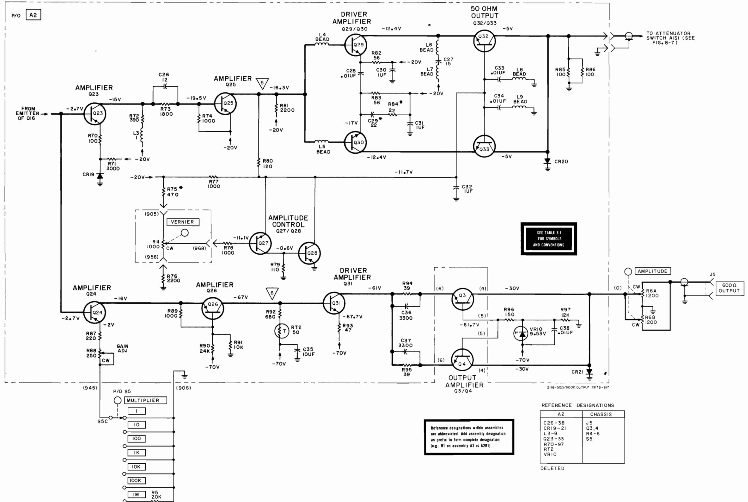
Figure 8-12. Output Circuitry Schematic
