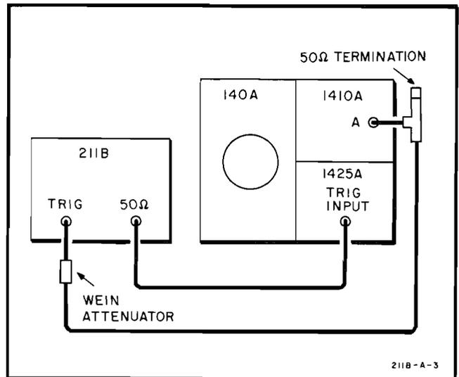
Figure 5-6. Trigger Output Test Setup
