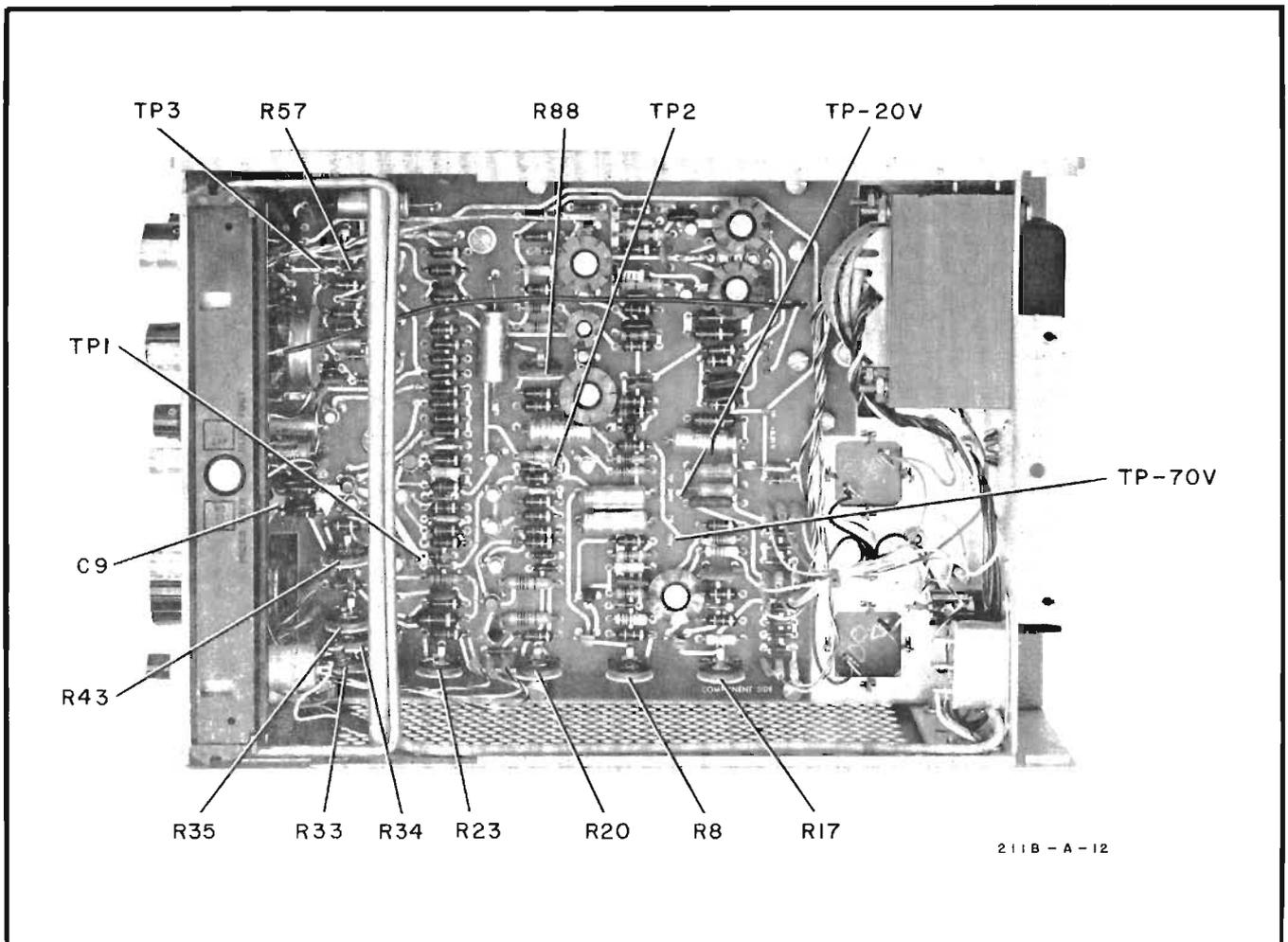
Figure 5-7. Component Adjustment Location
