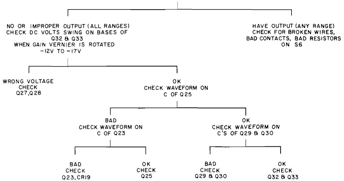
NO OR IMPROPER 600 OHM OUTPUT
