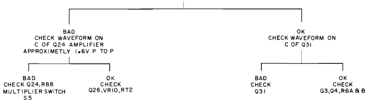
Figure 8-4. 50 Ohms-600 Ohms Output Troubleshooting Tree
