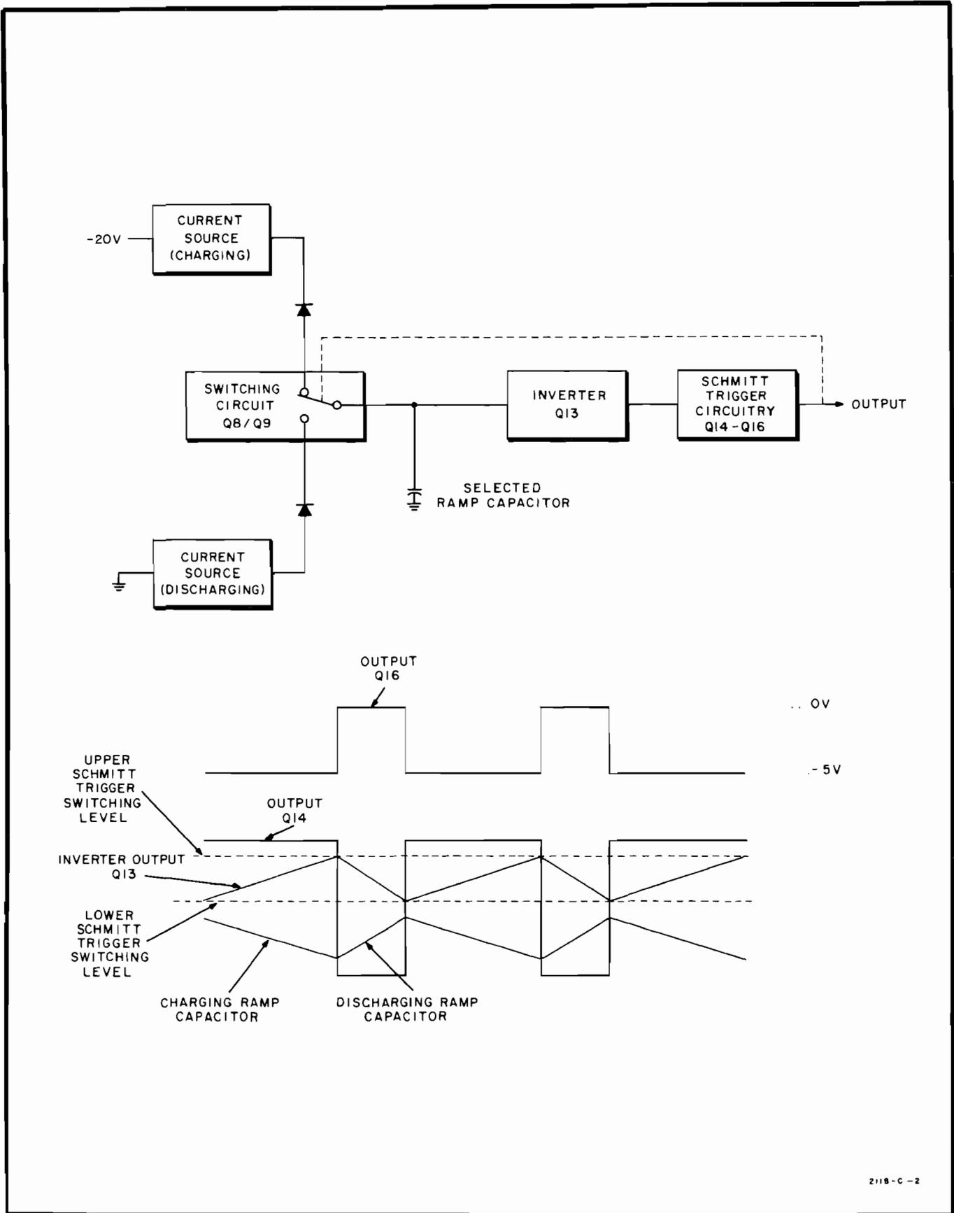
Figure 4-2. Schmitt Trigger Operation
