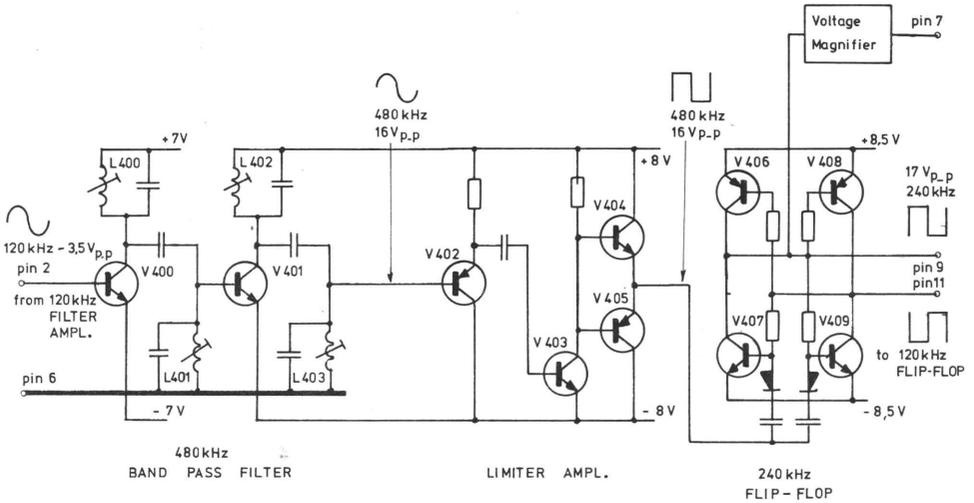
The purpose of this circuit is to create a 240 kHz square formed puls with a 180° phase difference for the two 120 kHz Flip-Flops which are used in the AC-DC Modulators to "beat" the 120 kHz Input Modulator signal down to a DC analog to the Input Level, and again to "Chop" the filtered DC back to 120 kHz as before.
