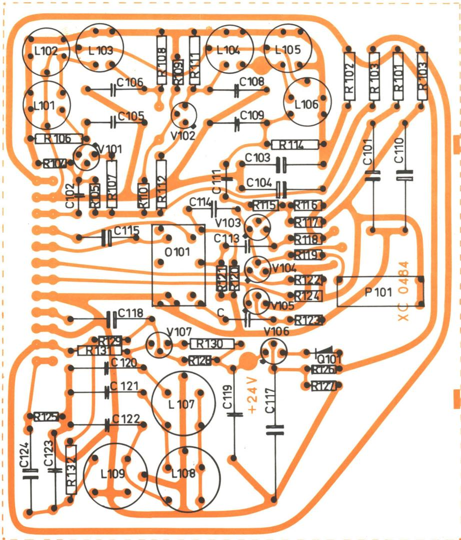
Input and 120 kHz Filter ZS 0168 – printed circuit XC 0484.
