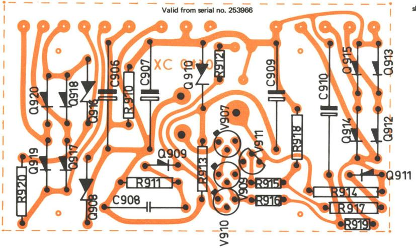
Negative Voltage Supply ZG 0017 - printed circuit XC 0490
