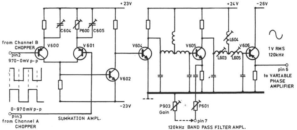
In this circuit the two chopped signals A and B are added together and fed through a 120 kHz Band Pass Filter.
