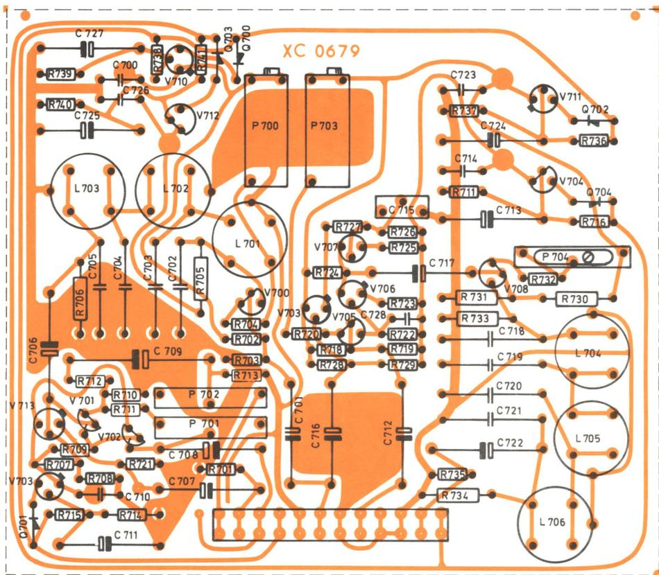
Rejection Ampl. LP Filter and Output Ampl. ZE 0086 – printed circuit XC 0679
