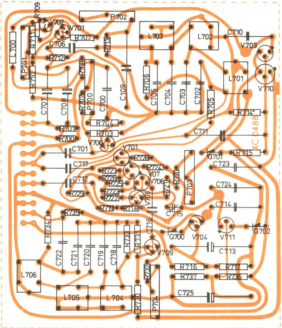
Rejection Ampl. LP Filter and Output Ampl. ZE 0029 – printed circuit XC 0488.
