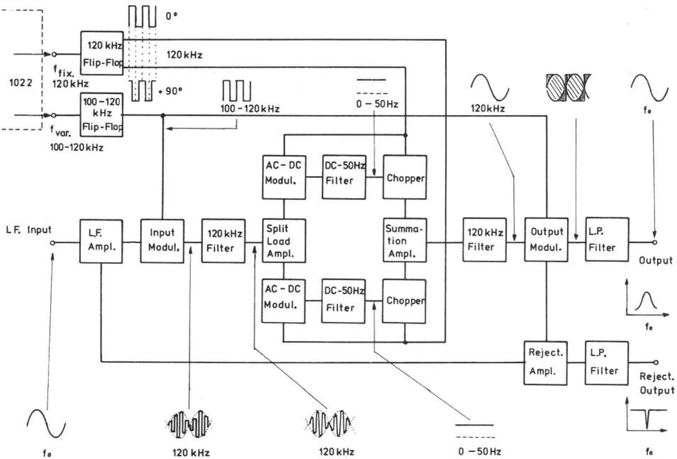
The Heterodyne Slave Filter Type 2020 is intended to be used together with a Beat Frequency Oscillator Type 1022 or 1024. The 1022 is a Heterodyne Oscillator having a fixed oscillator section of 120 kHz and a variable oscillator section of 100–120 kHz. A mixing of these two frequencies will give the low frequency output signal from 20 to 20000 Hz. Now if 1022 is tuned to a low frequency signal of 1 kHz the variable oscillator will have a frequency of 119 kHz.
