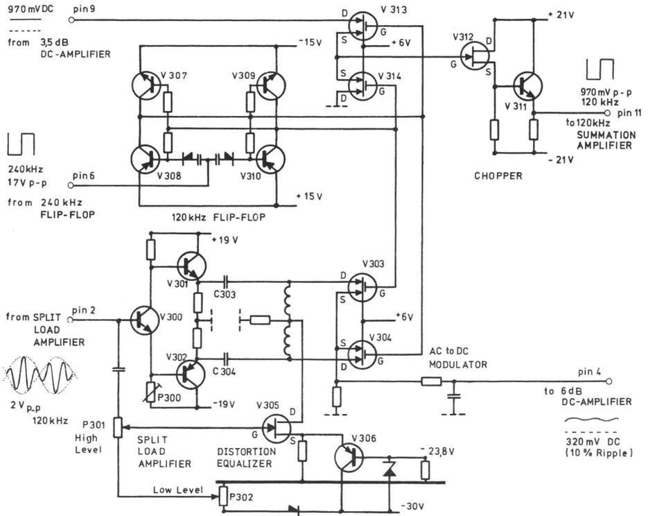
The AC to DC Modulators and Choppers ZM 0006 and ZM 007 are identical except for the Phase Lock arrangement, so only ZM 0007 will be mentioned.
