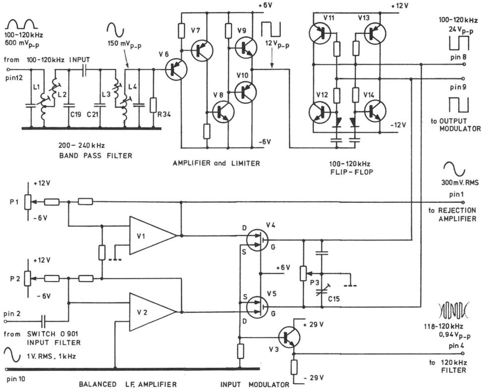
The Input Modulator consists of a 200–240 kHz Band Pass Filter with a succeeding pulseshaper which supplies squareformed pulses for a Flip-Flop circuit the output of which will have exactly the same frequency as the variable oscillator in the BFO 1022 (100–120 kHz).
