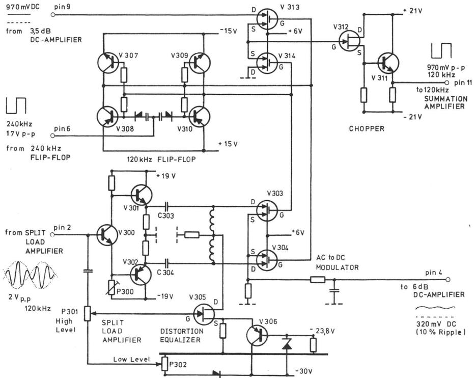
The AC to DC Modulators and Choppers ZM 0006 and ZM 0007 are identical except for the Phase Lock arrangement, so only ZM 0007 will be mentioned.
