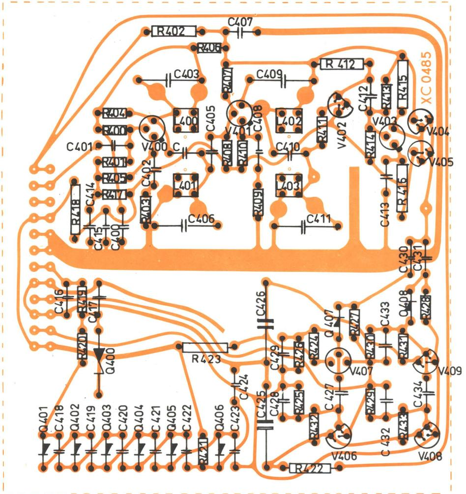
240 kHz square Wave Generator ZI 0003 – printed circuit XC 0485.
