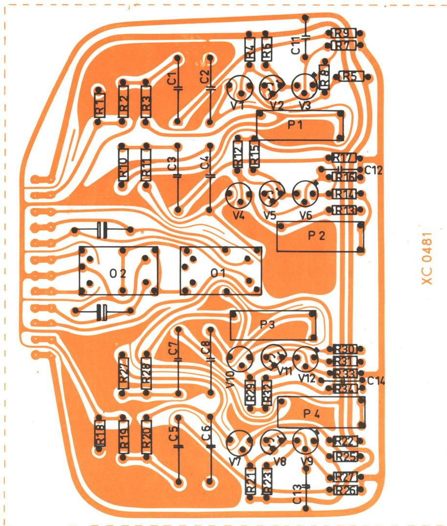
Main Filter 100 Hz ZT 0033 – printed circuit XC 0481
