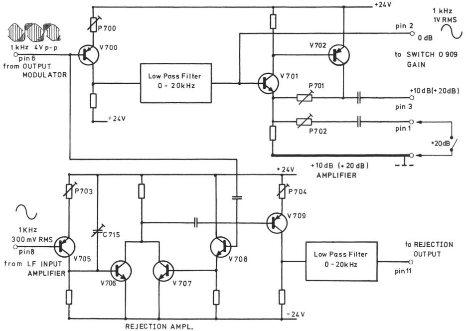
The input to V 700 is the filtered low frequency signal, which is applied to a 0 +10 and +20 dB output through a Low Pass Filter.
