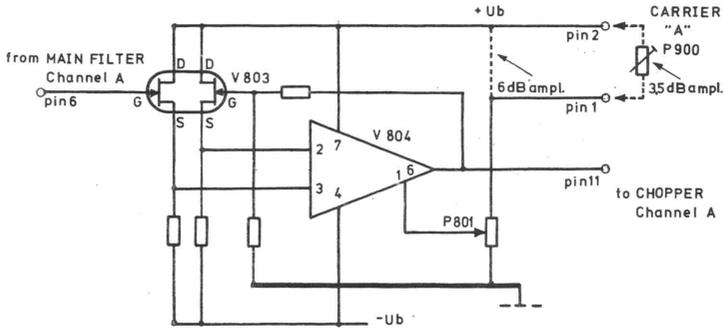
A simplified diagram of one D.C. amplifier is shown above (3.5 dB DC Ampl. channel A). The amplifier is designed as a differential amplifier with a positive and a negative supply voltage thus having 0 V DC on input and output in the balance condition without input signal.
