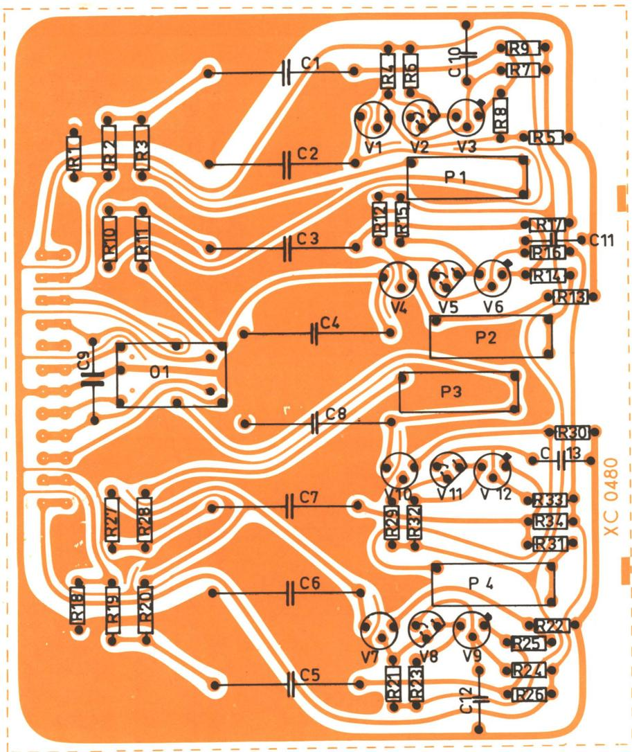
Main Filter 10 Hz ZT 0031 – 31.6 Hz ZT 0032 – printed circuit XC 0480.
