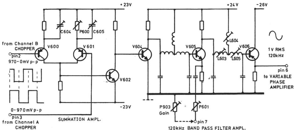
In this circuit the two chopped signals A and B are added together and fed through a 120 kHz Band Pass Filter. Here it is very important to have the correct voltage and phase applied to the base of V 602 and the adjustment is carried out as follows:
