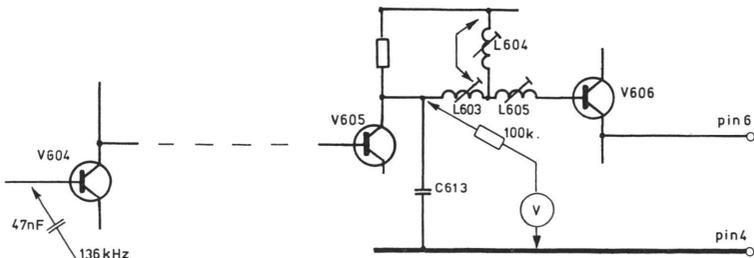
If adjustment is found necessary connect 136 kHz through a capacitor of 47 nF to the base of V 604, short connect L 604 and adjust L 603 to max voltage measured across C 613 with an electronic voltmeter with a series resistor of 100 k $\Omega$ .
