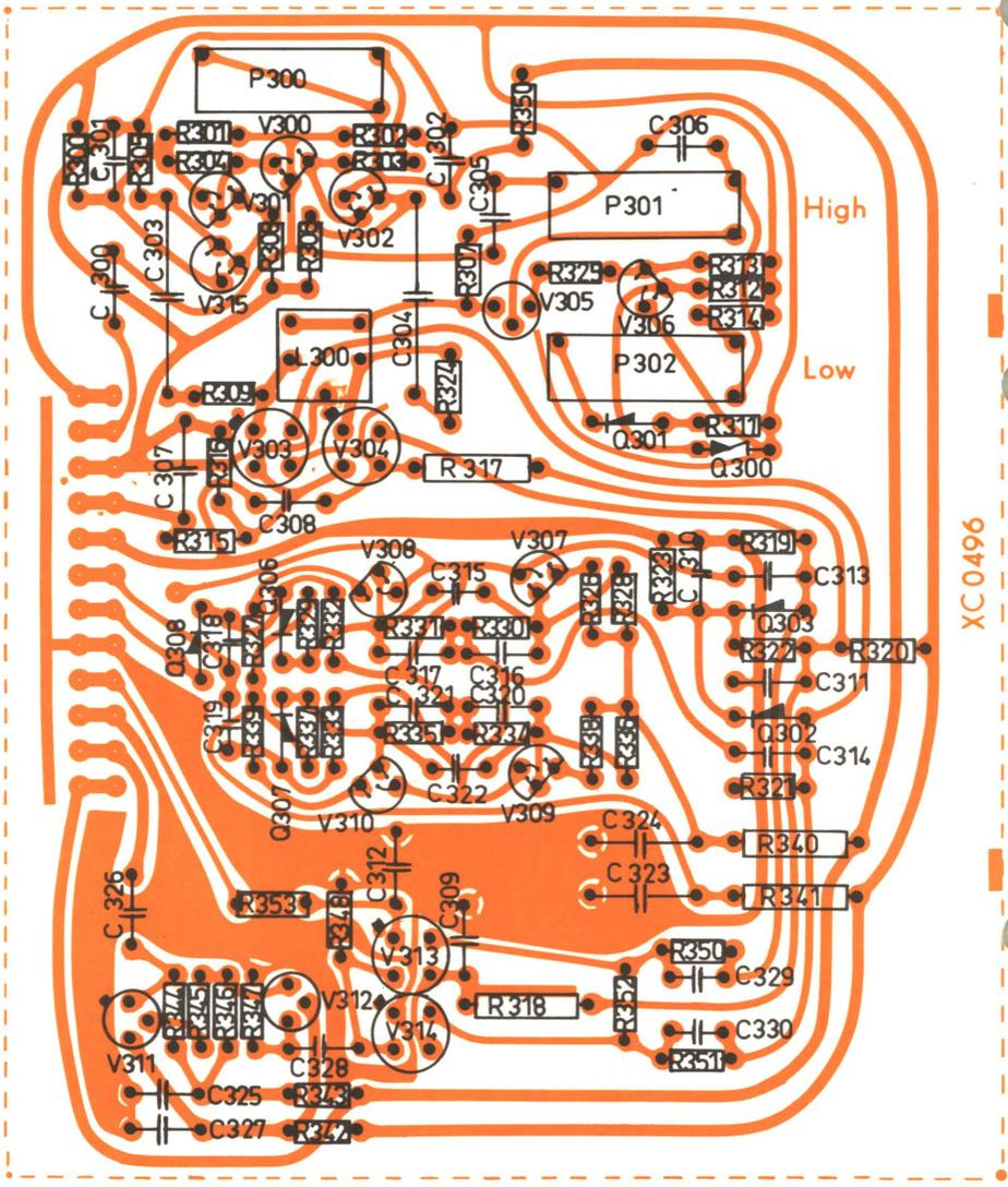
AC to DC Modulator and chopper ZM 0007 – printed circuit XC 0496.
