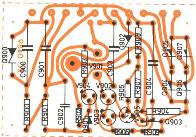
Positive Voltage Supply ZG 0016 - printed circuit XC 0489
