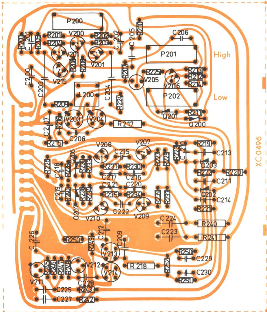
AC to DC Modulator and chopper ZM 0006 – printed circuit XC 0496.
