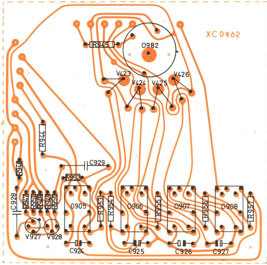
Filter Band Width OE 0006 – printed circuit XC 0495
