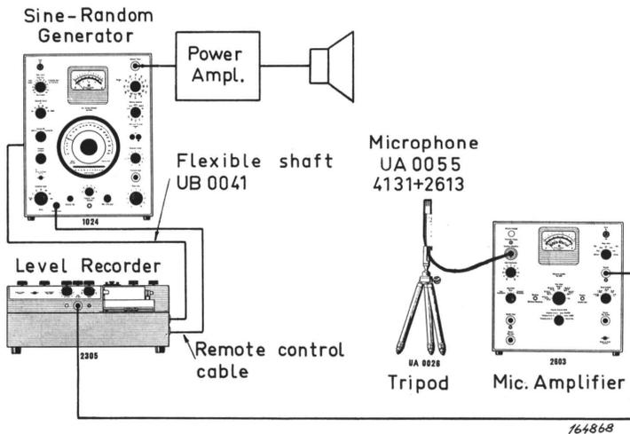
Fig. 4.16. Measuring equipment for the automatic recording of reverberation time.
