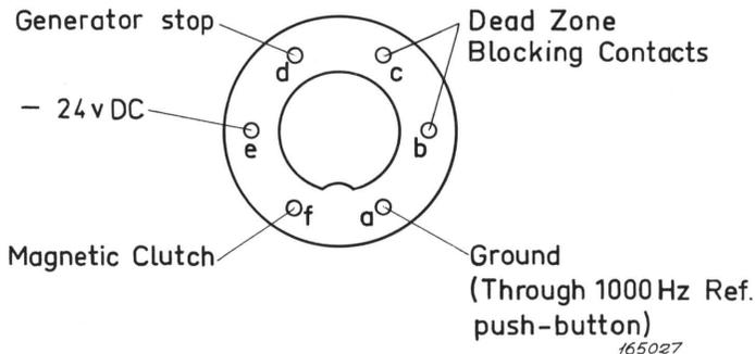
Fig. 3.4. REMOTE CONTROL socket, viewed internally.
