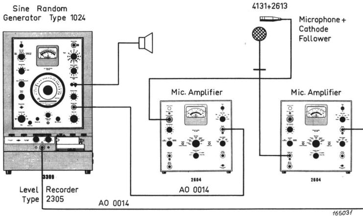
Fig. 4.6. Measuring set-up for automatic recording of the frequency response of microphones.
