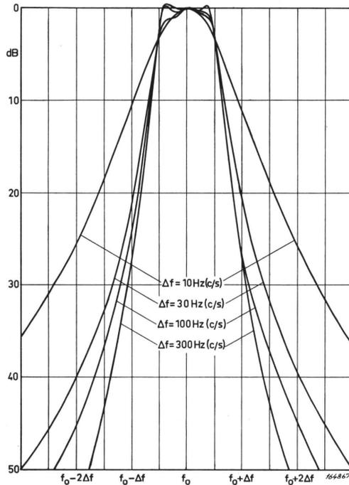
Fig. 1.2. Typical Spectrum characteristics of the various narrow noise bands.
