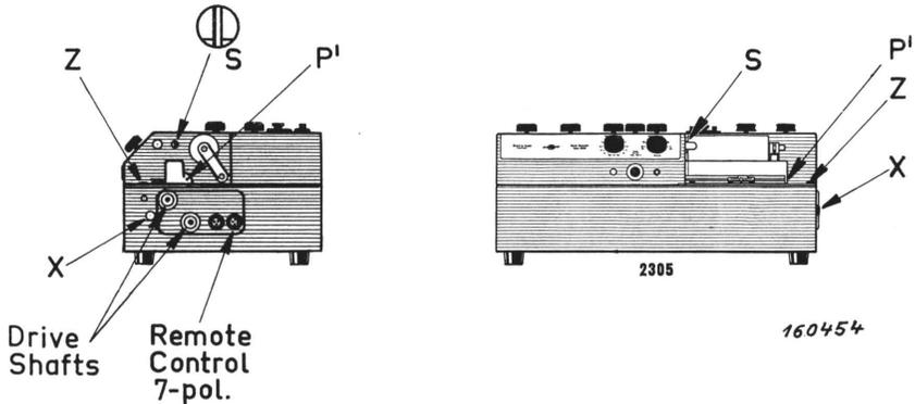
Fig. 3.3. Front and side views of the Level Recorder.
