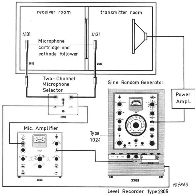
Fig. 4.14. Measuring set-up for sound insulation measurements.
