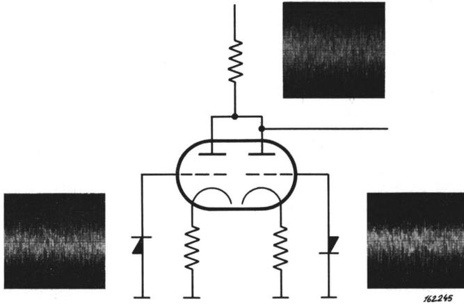
*Fig. 1.6. Schematic illustration of the noise source arrangement.*
