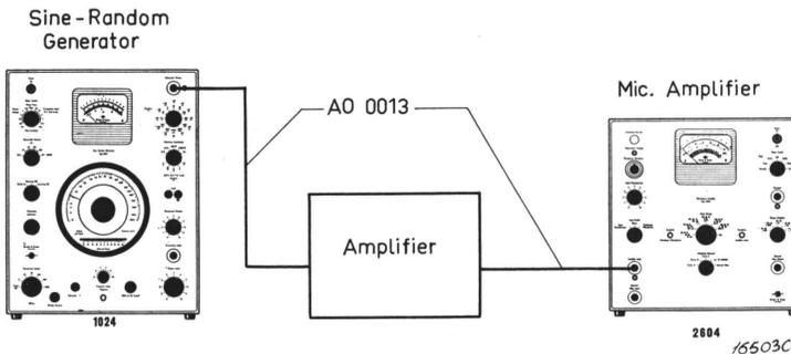
Fig. 4.4. Measurement of gain in an AF amplifier.
