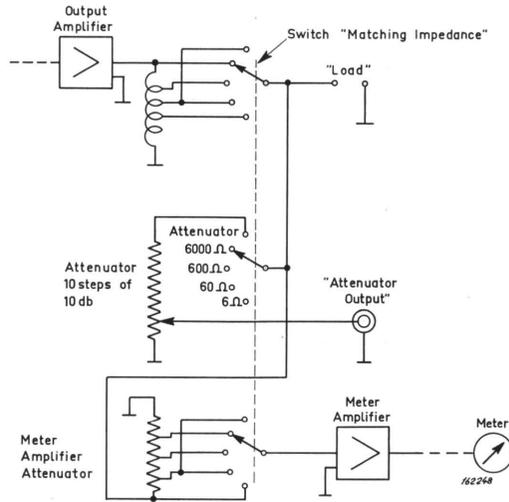
Fig. 1.4. Schematic diagram of the Generator's output circuitry.
