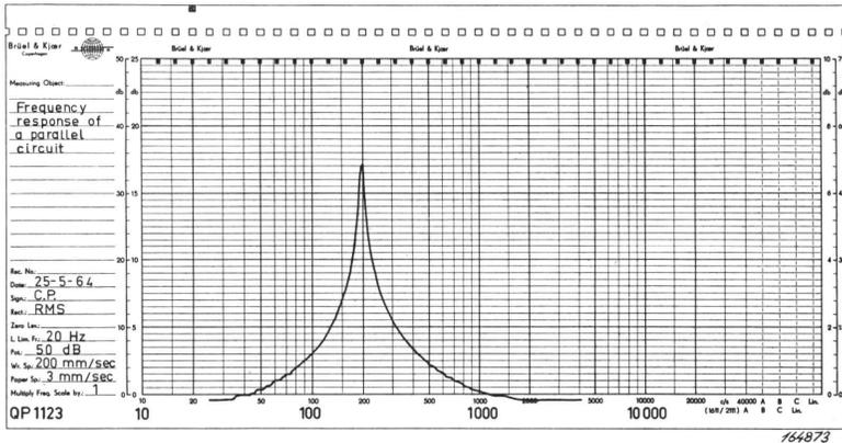
Fig. 4.2. Frequency Response of a four-terminal network.
