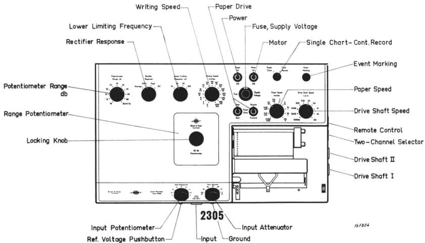
Fig. 3.2. Level Recorder Type 2305 viewed from above.
