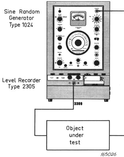
Fig. 3.1. External electrical connections when using Automatic Frequency Response Recorder Type 3309. If necessary an amplifier can be used between the test object and the Level Recorder.
