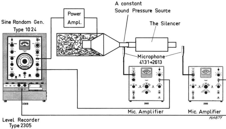
Fig. 4.12. A set-up used for measurements on silencers.
