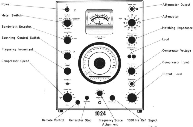
Fig. 2.1. Sine Random Generator Type 1024 front panel.
