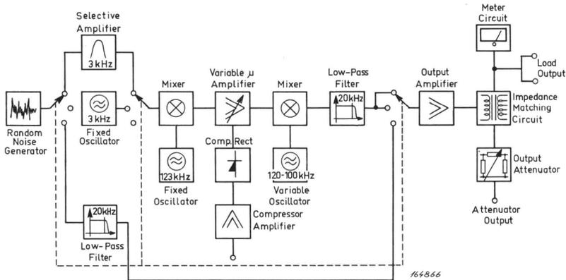
Fig. 1.1. Block diagram of the Sine-Random Generator.
