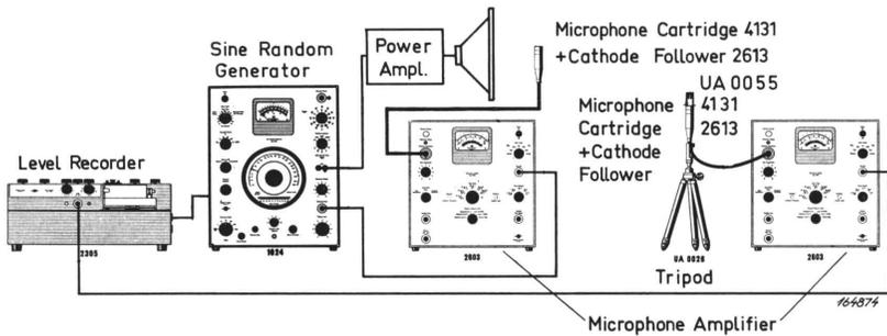
*Fig. 4.21. Measuring arrangement for sound distribution analysis.*
