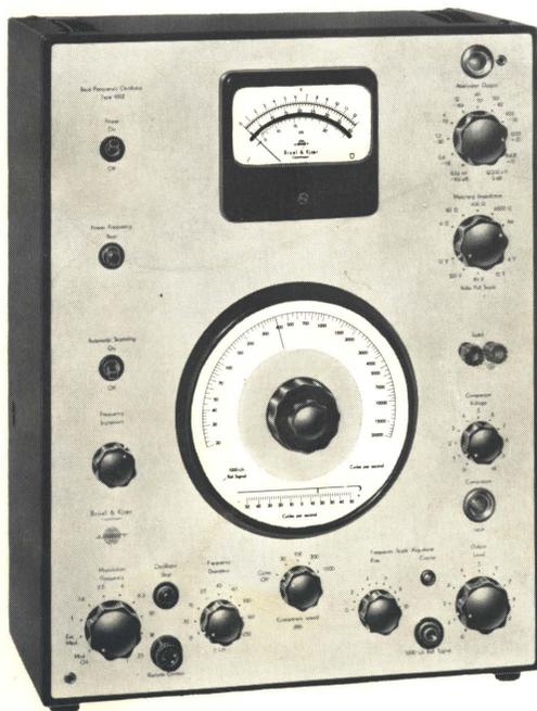
A beat frequency oscillator covering the range 20 to 20000 c/s. The apparatus is designed to meet the numerous requirements of a signal source for audio frequency work. It is excellently suited both for electrical and electroacoustical measurements, as well as for acoustic research.
